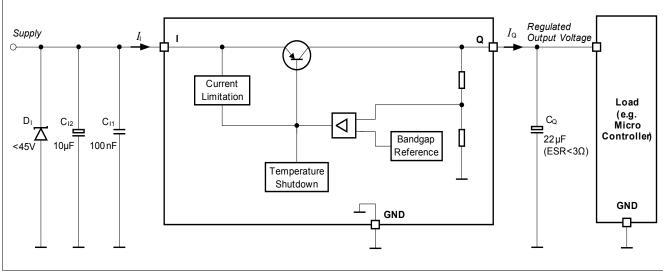
Figure 4 Application Diagram
