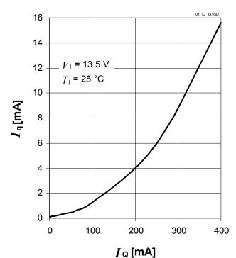
Current Consumption  $I_{\rm q}$  versus Low Output Current  $I_{\rm Q}$
