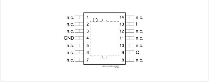
Figure 3 Pin Configuration (top view)
