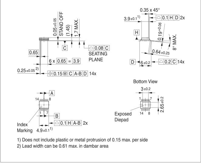
Figure 7 PG-SSOP-14 exposed pad
