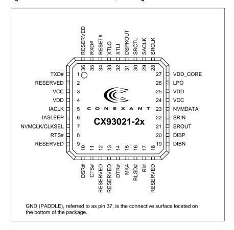
Figure 3-2. CX93021-2x Modem 36-Pin QFN Pin Signals
