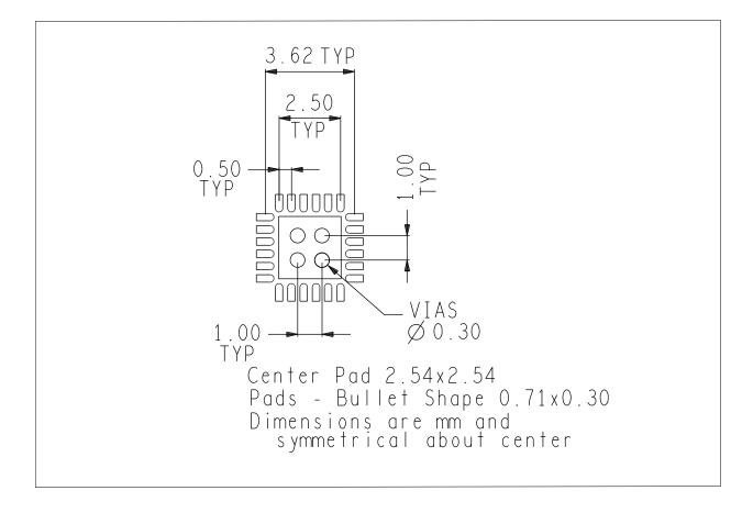
Figure 5-3. Recommended Surface Mount Land Pattern for 16-Pin QFN
