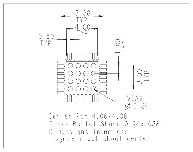
Figure 5-2. Recommended Surface Mount Land Pattern for 24-Pin QFN
