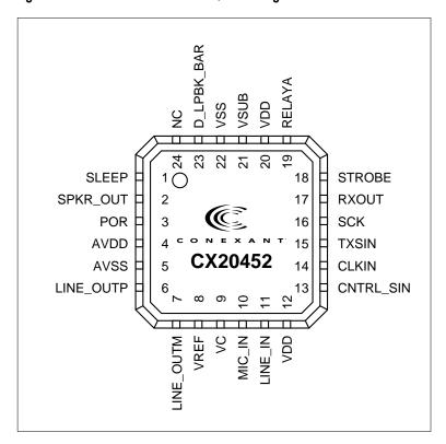
Figure 3-6. CX20452 Codec 24-Pin QFN Pin Signals
