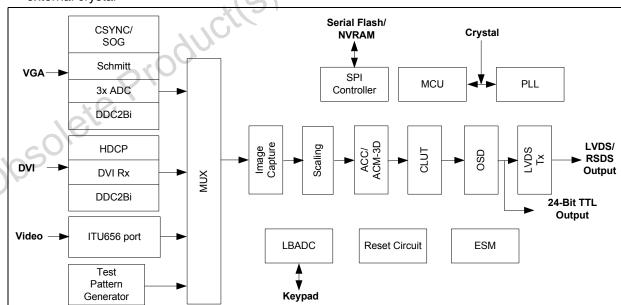
Note: ITU656 video input port is available only with LVDS and TTL panel interface and is not available for RSDS application.
