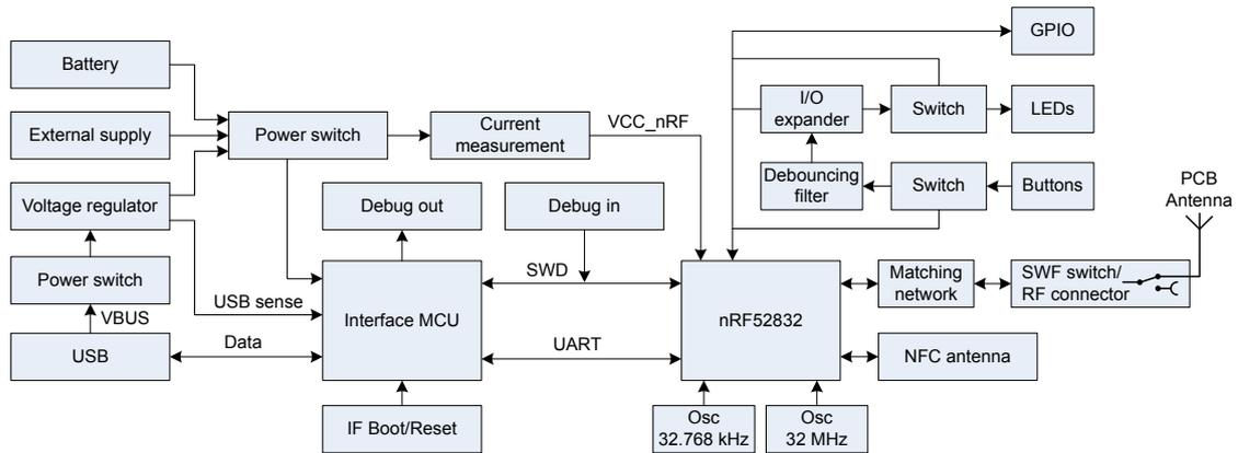
Figure 5: nRF52 Development Kit board block diagram
