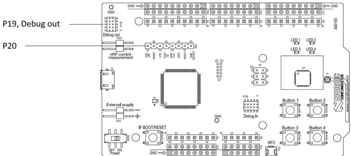
Figure 23: Debug output connector
