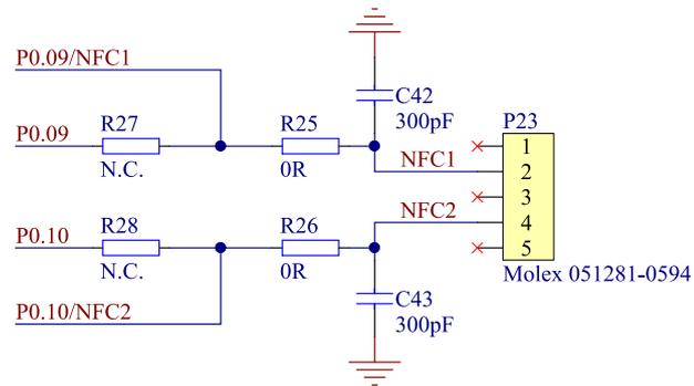
Figure 25: NFC input schematic
