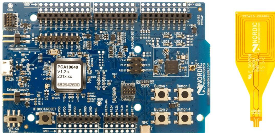
Figure 1: nRF52 Development Kit board (PCA10040) v1.2.x and NFC tag
