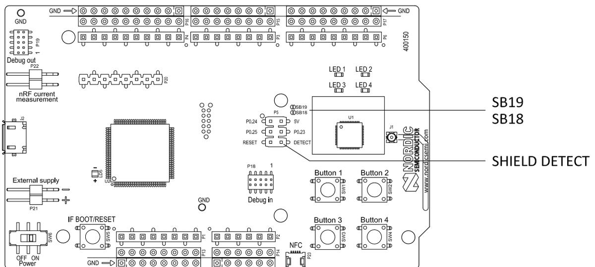
Figure 14: Enable or disable I/Os for Arduino standard
