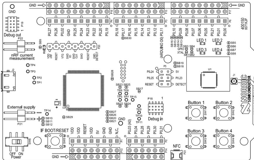
Figure 3: nRF52 Development Kit board top view
