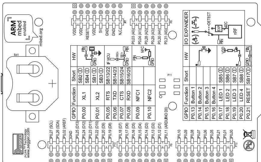
Figure 4: nRF52 Development Kit board bottom view
