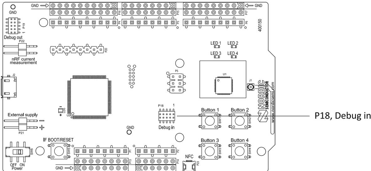
Figure 22: Debug input connector
