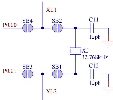
Figure 17: 32.768 kHz crystal and SB1 to SB4 schematic
