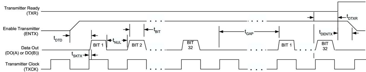
Figure 10: Transmitter Timing Diagram
