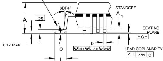
Figure 14: 44 Lead 13.90mm PQFP Mechanical Outline (44 PQFP)
