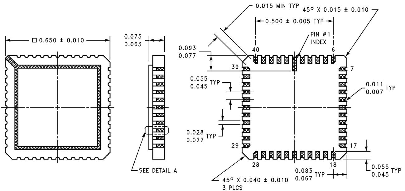
Figure 16: 44 Lead CLCC Mechanical Outline (44 CLCC)
