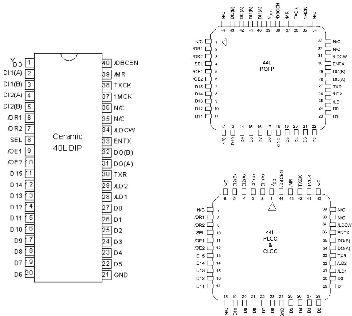
Figure 11: Terminal Connections
