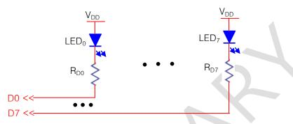
In the case of 2-color LED drive M1, M2 and D0~D7 must be equipped as below figure, and write the 'par\_output\_mode' bit of 'global\_ctrl2' register as '0' and the 'pwm\_sel' bit of 'global\_ctrl2' register as '1'. M1 and M2 have alternatively high and low pulse and the pulse duty is 50%. During M1 is high M2 is low, D0~D7 has 1pwm pulse of each D0~D7. During M1 is low M2 is high, D0~D7 has 2pwm pulse of each D0~D7.
