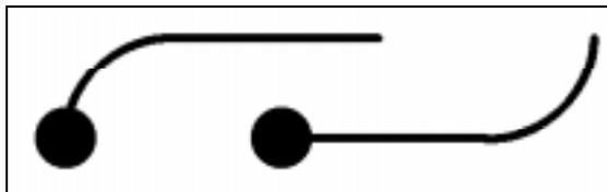
*a via is placed automatically when you change layers*
