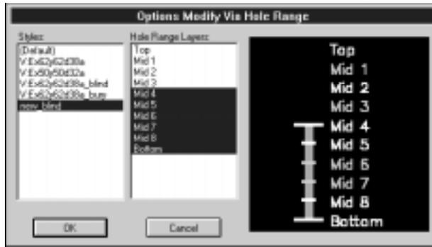
Set your new via current and place one. Toggle to each layer and redraw to verify your construction. Note that you “see through” to layer Mid4 when the top layers are current, since no pads are defined for those layers. The pads should look like this on Mid4, Mid5 - Mid8, and Bottom:
