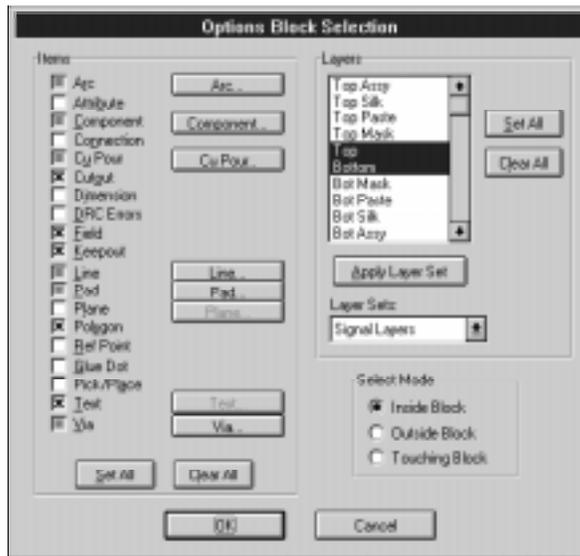
Try selecting all text on your current Schematic sheet or PCB design. Click the **Clear All** button and then enable only the **Text** checkbox. In PCB, click **Set All** to enable all layers; block selection looks for items only on enabled layers. Choose the **Outside Block** radio button then click **OK**. Be sure you are in Select mode, then click and drag to define a small selection box, making sure you avoid all text. Practice choosing items inside, outside, and touching a block.
