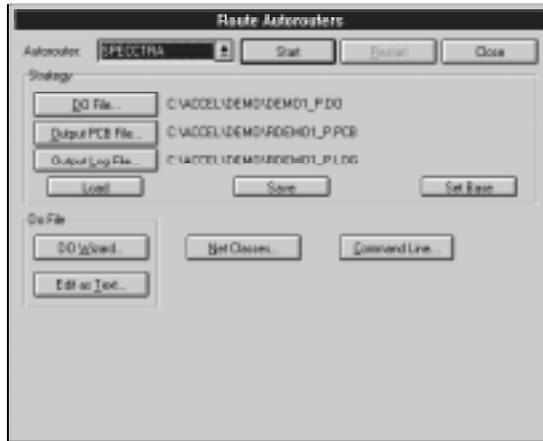
The SPECCTRA autorouters are controlled by router commands supplied in a DO File. Click the **DO Wizard** push-button for help in creating a command file. Select various commands from the drop down **DO Commands** list box and notice the right portion of the dialog changes to display valid arguments for each selected command. This context-sensitive dialog helps ensure your command arguments are valid and syntactically correct.
