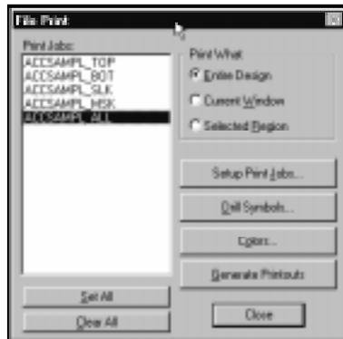
We designed this dialog box to make it easy to examine or change an existing job, or to create a new one. Notice you can print the entire database, the contents of the current window, or the selected region. The push buttons on the right are positioned in the order that you would use them. Click **Setup Print Jobs**. Here you set up your print options and items to be including in the output.
