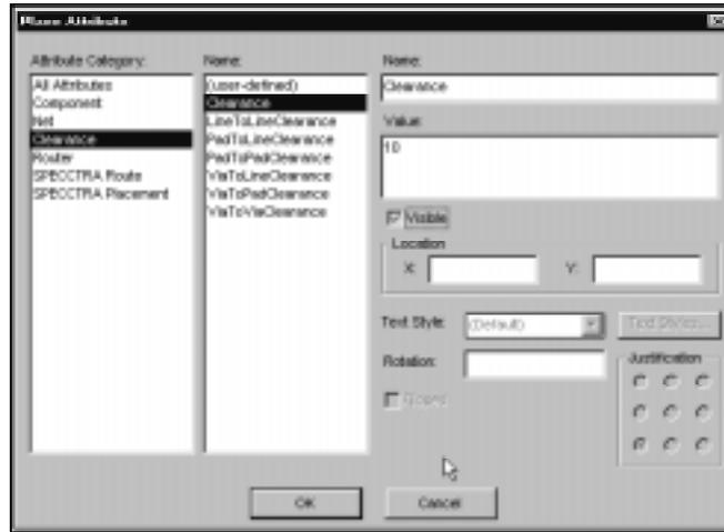
Press **OK** and you will see the newly added entry in the list. Net attributes are transferred in the ACCEL EDA netlist from the schematic to the PCB, where many are used for operations such as DRC, pin and gate swapping, and routing. Press **OK** and then **Close** to exit the dialogs.
