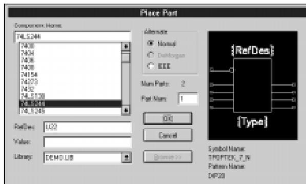
Pick 74LS244 from the **Component Name** list or start typing in the box and see how the list automatically scrolls to display parts having the given prefix. Notice **Num Parts** is set to 2, indicating two of these parts fit into one component package. Click **OK**.
