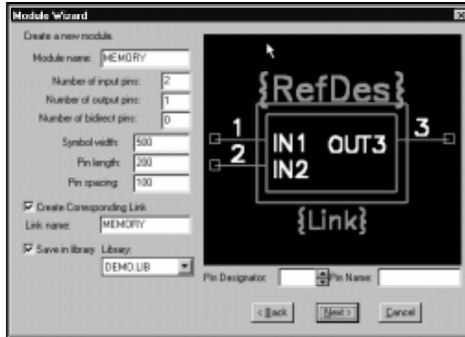
Press **Next >** and then enter MEMORY as the name of the sheet on which the links (and your sub-circuit logic) will be placed.
