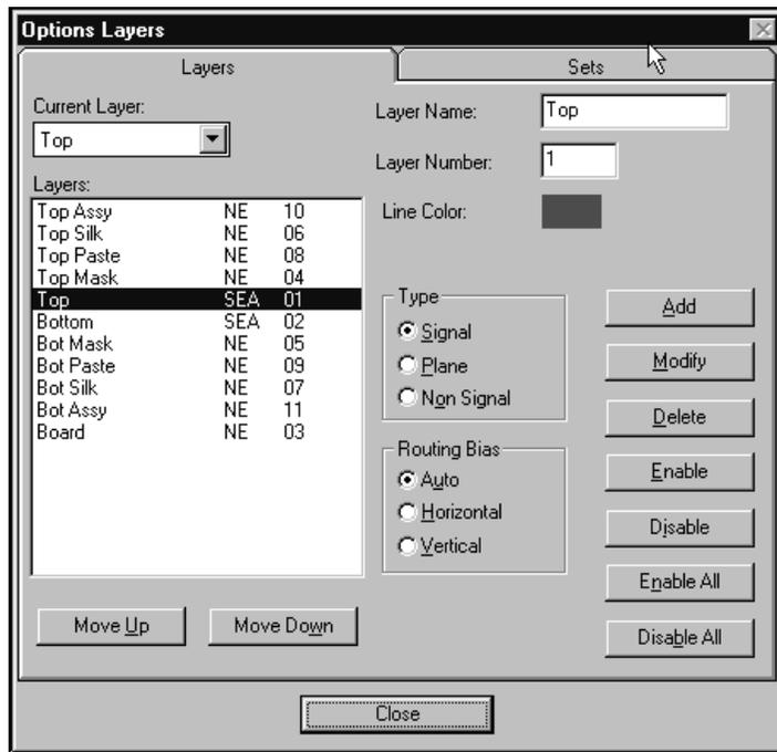
For **non signal** silk layers, the layer mapping is to Top Silk or Bottom Silk. The board outline should map to the Board layer:
