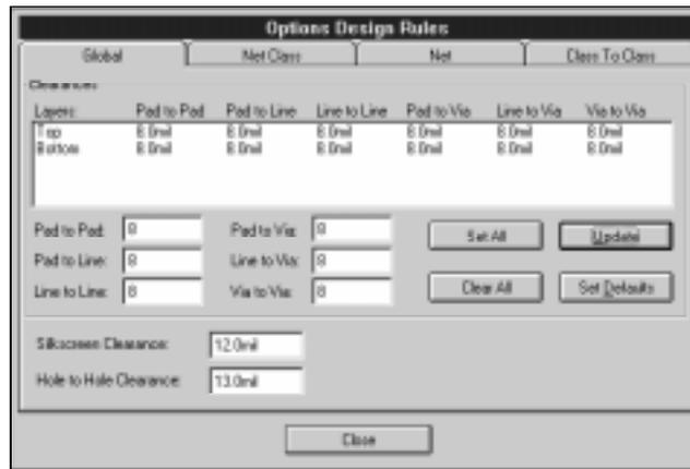
Notice the tabs reflect the hierarchy of design rules. Rules at all levels of the hierarchy may be transferred from the schematic to the PCB design in the netlist. Turn to the Schematic Design Session for a detailed description of the design rule hierarchy. The information is not repeated here.
