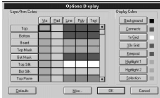
setting up layers Choose the Options Layers command and notice that the range of options includes adding, deleting, ordering, and enabling layers for your design. The existing design layers are listed in the **Layers** list box. ACCEL EDA allows up to 99 layers; 11 *predefined* and 88 user-defined layers.
