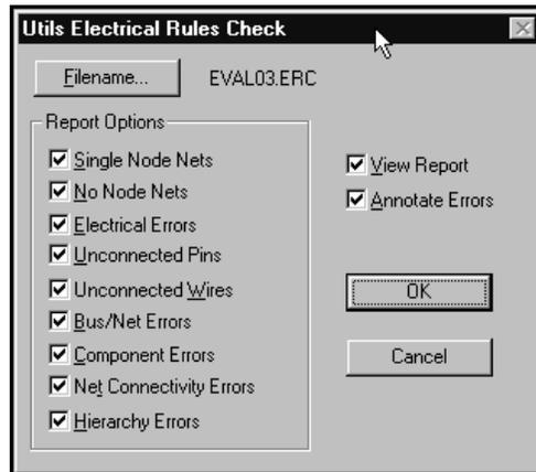
The ERC report is opened using the File Viewer specified in Options Configure. Window's Notepad is the default. Reports are viewed, edited, or printed from that utility. Several errors will be reported including missing input and output pins, bus violations, unconnected pins, and a single node net. Toggle back to your design and notice that indicators have been placed.
