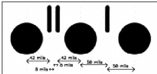
Setting a non-uniform, relative grid can be done directly on the Status line. However, because we will also be changing the relative grid origin, we need to bring up the Options Grids dialog. Choose this command and click **Relative Mode**. Type **42 8 8 42** in the **Grid Spacing** box with the values separated by spaces. Click **Add**. If you are working in mms, unit overrides must be typed for each value (e.g., 42mil 8mil 8mil 42mil).
