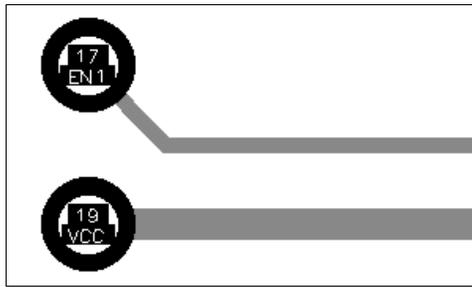
12. Continue practicing with orthogonal modes, placing one or two traces between pads, toggling between layers, and creating t-routes by terminating a trace on another one in the same net. Don't worry if you fall short -- DRC warns of incomplete connections. When you route directly to the destination pad a diamond shape appears, indicating routing is complete with a zero length connection.
