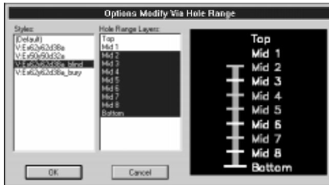
When manually routing from one layer to another, ACCEL EDA will alert you if you try to insert a via between layers that the current via style does not support. For instance, you'll be warned if you try to route from the Top to Bottom layers when our blind via style is current.
