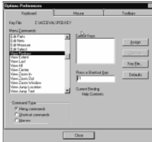
Assigning *F1* to Redraw would delete the current assignment. Instead, press *F3* (which has no other assignment) and click the **Assign** button to bind *F3* to the command.
