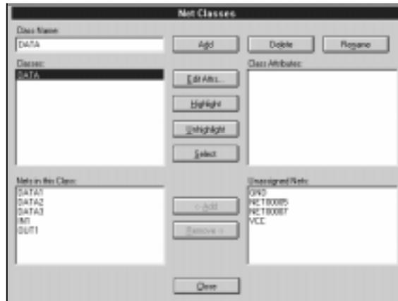
Select the DATA\* nets in the **Unassigned Nets** box (use the *Shift* key to select a range, or the *Ctrl* key to select individual nets) and press the **<-Add** button. Similarly, add the IN1 and OUT1 nets to the class. Click **Edit Attrs** to present the familiar Attributes dialog box. Assign a **Clearance** attribute of 8 to the class.
