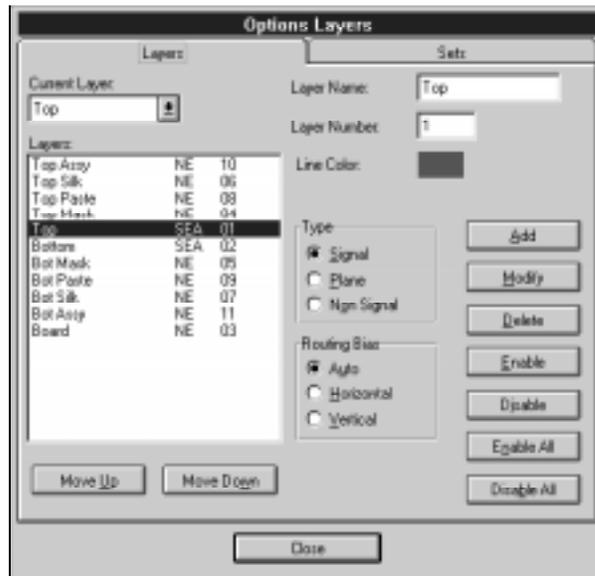
The letters between the layer name and layer number in the **Layers** box signify (in the case of the Top layer) **S** for Signal layer, **E** for Enabled, and **A** for a Routing Bias set to Auto. Other codes you will see are **P** for Plane, **N** for Non-Signal, **D** for Disabled, **H** for Horizontal, and **V** for Vertical.
