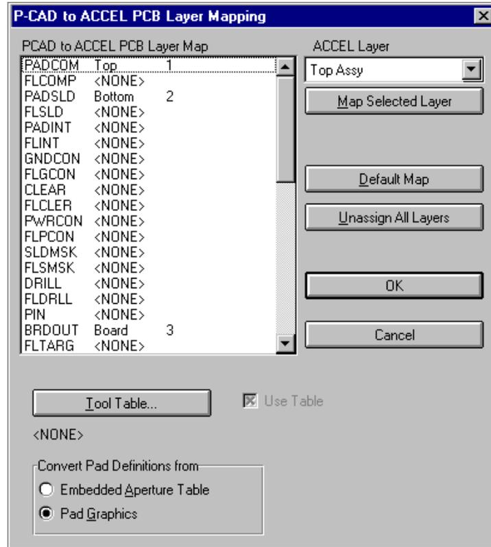
**P-CAD to ACCEL PCB Layer Map:** Displays the P-CAD layer mapping assignments. A <NONE> next to the P-CAD layer name indicates that PCB will ignore data on that layer. A typical layer assignment looks like this:
