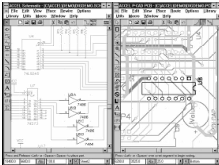
Two highlight colors are used interchangeably. Highlight the component a second time, and notice the color change. Next, select a net by selecting one trace segment, clicking right and choosing **Select Net**. Highlight these items and notice the corresponding wires in the Schematic are highlighted.
