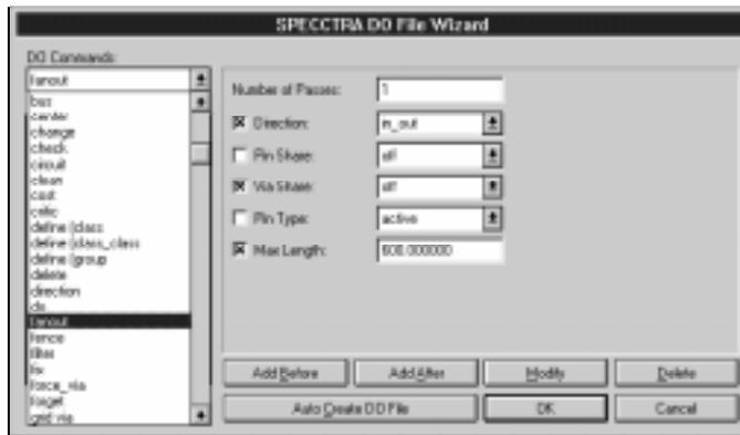
You add a new router command to the DO File by selecting the command from the list box, filling in the arguments in the right portion of the dialog, and pressing **Add Before** or **Add After**. The new entry is added to the **DO File** list box.
