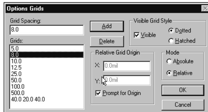
Notice you can also control the grid visibility and style, delete a grid, and define the relative origin from within the dialog.
