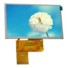
4.3 Inch 480 (RGB) X272 TFT LCD Module LCD Display with Contrast Ratio 500
