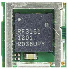
RF3161 (Quad band power amplifier module)
