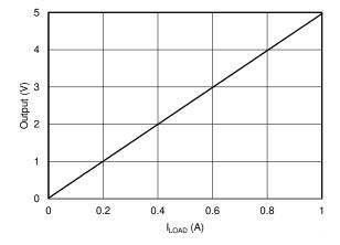
Figure 8-2. Low-Side, Current-Sense Transfer Function
