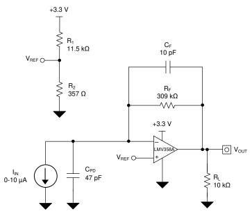
Figure 8-3. Single-Supply Photodiode Amplifier Circuit
