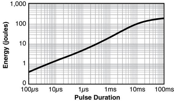
Limit of acceptance is a shift in resistance of less than 1% from the initial value. 100 joule Energy rating is for 10 mSec pulse width; for shorter pulses energy rating has to be derated according to above rating chart
