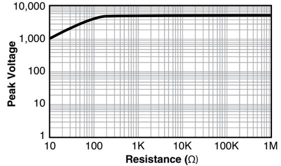
TRHE are tested in accordance with IEC61000-4-5, waveform 1.2/50ms, 10 pulses applied. Limit of acceptance is a shift in resistance of less than 1% from the initial value.
