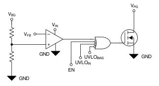
Figure 29. Simplified PG Circuit
