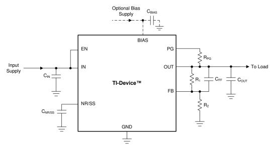
Figure 30. Adjustable Operation
