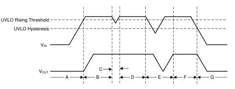
Figure 31. Typical UVLO Operation
