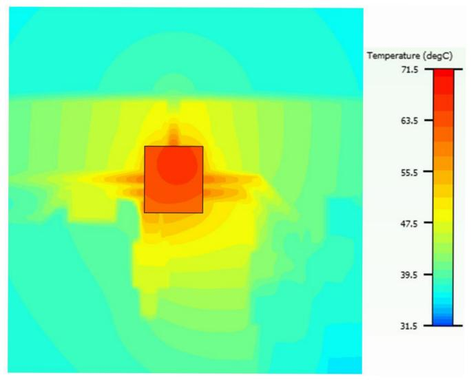
Figure 39. PCB Thermal Gradient
