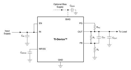
Figure 40. Typical Application for a 0.9-V Rail
