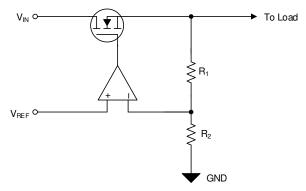
NOTE:  $V_{OUT} = V_{REF} \times (1 + R_1 / R_2)$ .
