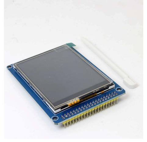
3.2 inch 320x240 Touch TFT LCD Display with SD Card Slot Pen
