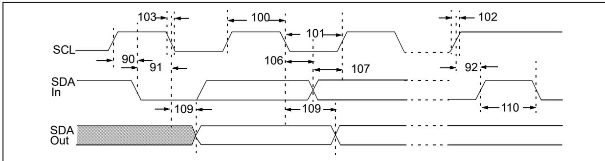
**FIGURE 1-3:** I<sup>2</sup>C Bus Timing Waveforms.
