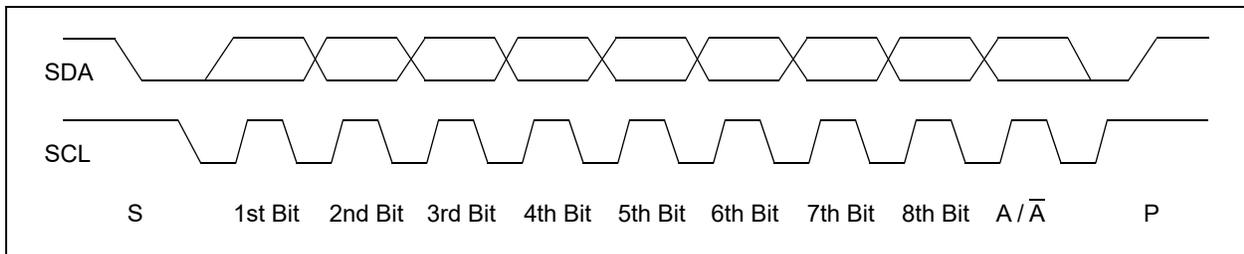
**FIGURE 6-7:** Typical 8-Bit I<sup>2</sup>C Waveform Format.
