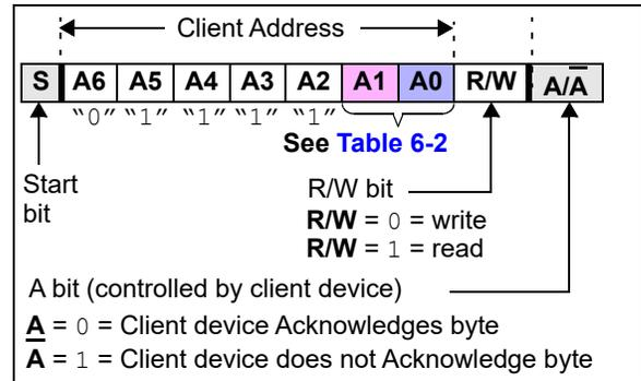
**FIGURE 6-9:** Client Address Bits in the I<sup>2</sup>C Control Byte.
