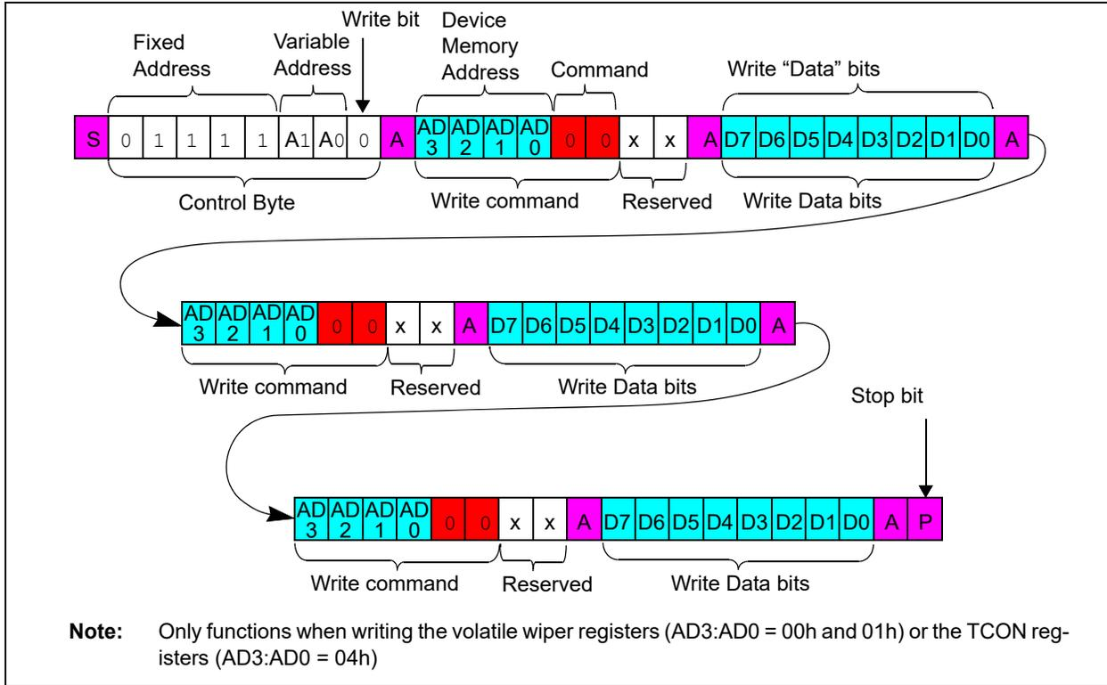
**FIGURE 7-3:** I<sup>2</sup>C Continuous Volatile Wiper Write.
