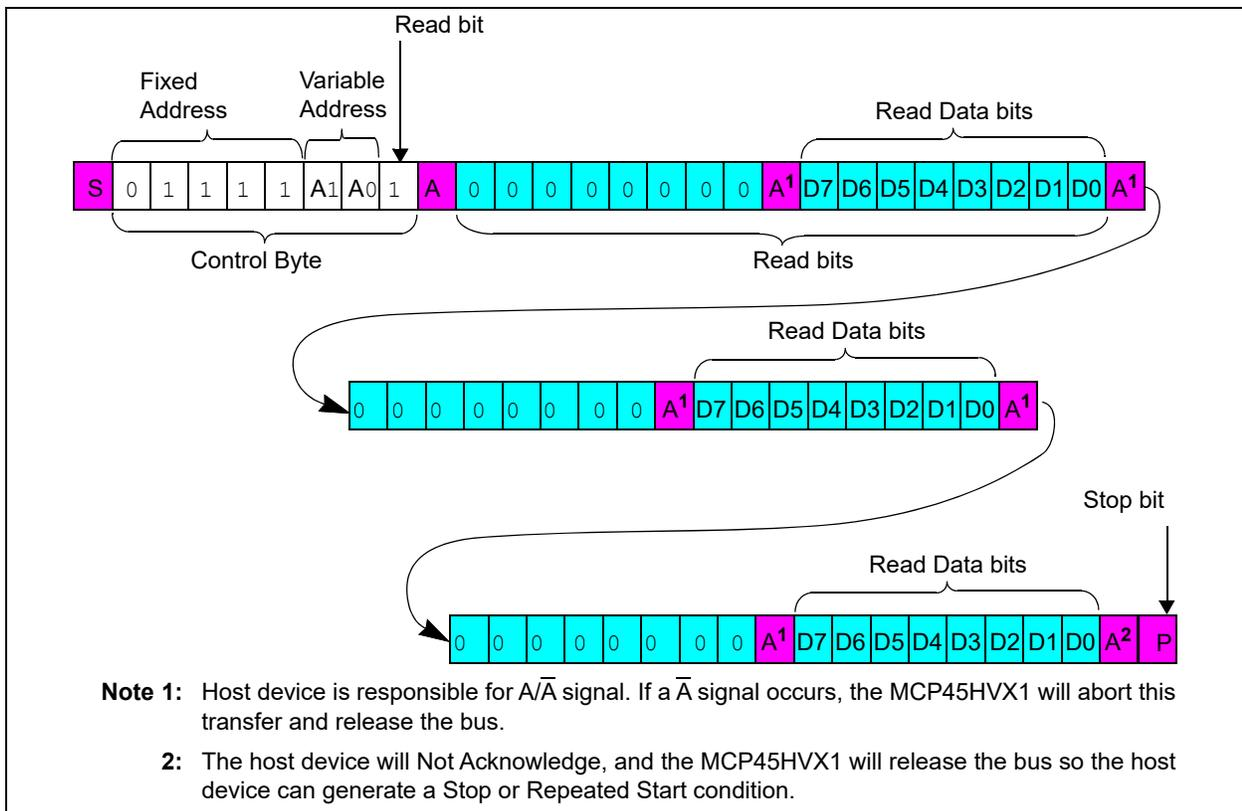
**FIGURE 7-6:** I<sup>2</sup>C Continuous Reads.
