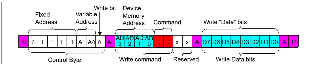
**FIGURE 7-2:** I<sup>2</sup>C Write Sequence.
