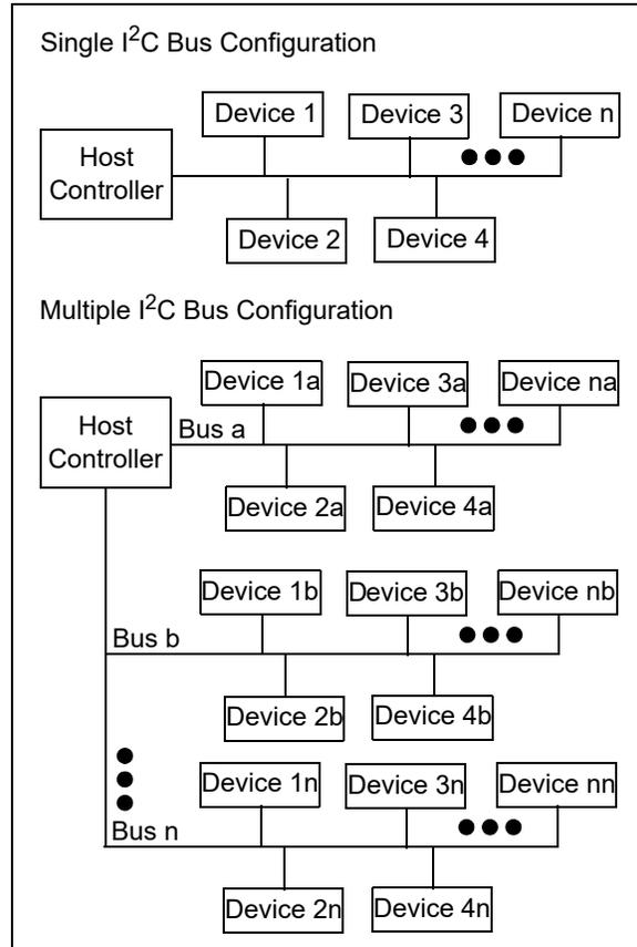
**FIGURE 8-11:** Typical Application I<sup>2</sup>C Bus Configurations.
