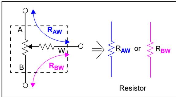
**FIGURE 5-8:** Rheostat Configuration.
