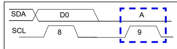
**FIGURE 6-4:** Acknowledge Waveform.
