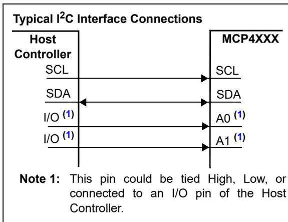
**FIGURE 6-1:** Typical I<sup>2</sup>C Interface Block Diagram.
