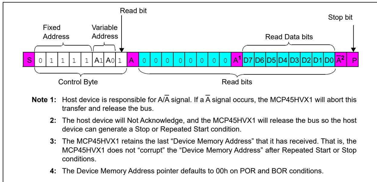
**FIGURE 7-4:** I<sup>2</sup>C Read (Last Memory Address Accessed).
