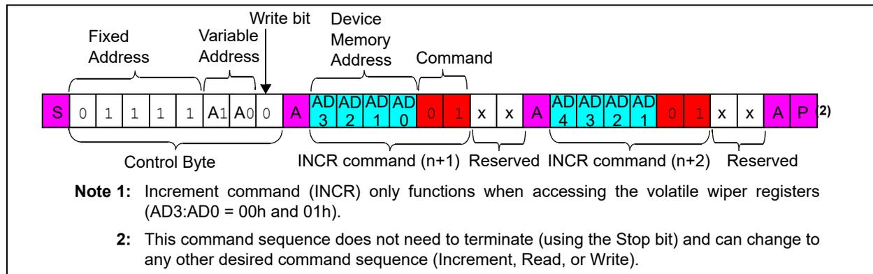
**FIGURE 7-7:** I<sup>2</sup>C Increment Command Sequence.
