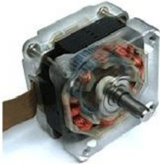
A stepper motor (or step motor) is a brushless DC electric motor that divides a full rotation into a number of equal steps. The motor position can then be commanded to move and hold at one of the steps without any feedback sensor (an open-loop controller), as long as the motor is carefully sized to the application.
