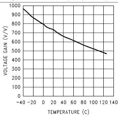
Figure 11. Error Amp Voltage Gain vs Temperature
