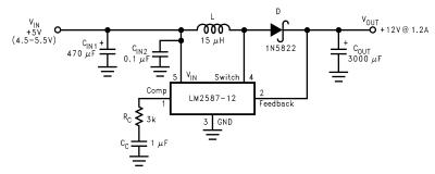
By adding a small number of external components (as shown in Figure 16), the LM2587 can be used to produce a regulated output voltage that is greater than the applied input voltage. The switching waveforms observed during the operation of this circuit are shown in . Typical performance of this regulator is shown in .
