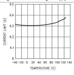
Figure 5. Current Limit vs Temperature
