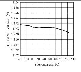
Figure 2. Reference Voltage vs Temperature
