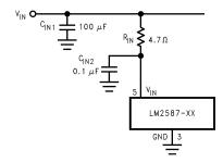
Figure 60. Input Line Filter
