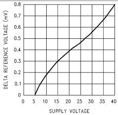
Figure 3. ΔReference Voltage vs Supply Voltage
