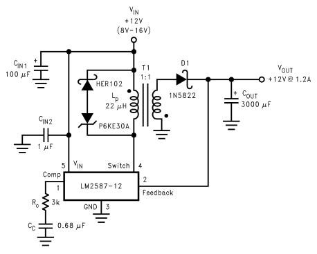
Figure 15. 12-V Flyback Regulator Design Example
