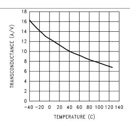
Figure 8. Switch Transconductance vs Temperature
