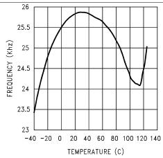
Figure 12. Short Circuit Frequency vs Temperature
