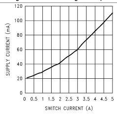
Figure 4. Supply Current vs Switch Current
