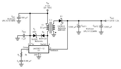
Figure 24. Single-Output Flyback Regulator
