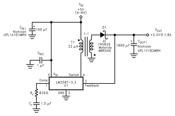
Figure 22. Single-Output Flyback Regulator
