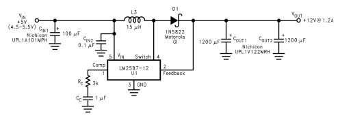
Figure 18. 5-V To 12-V Boost Regulator
