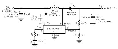
\*The LM2585 will require a heat sink in these applications. The size of the heat sink will depend on the maximum ambient temperature. To calculate the thermal resistance of the IC and the size of the heat sink needed, see
