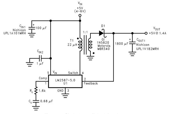
Figure 23. Single-Output Flyback Regulator
