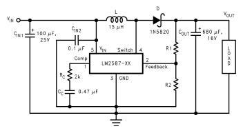
$C_{IN1}$ —100 μF, 25V Aluminum Electrolytic  $C_{IN2}$ —0.1 μF CeramicL—15 μH, Renco #RL-5472-5D—1N5820 $C_{OUT}$ —680 μF, 16V Aluminum Electrolytic  $C_{C}$ —0.47 μF Ceramic  $R_{C}$ —2kFor 12V Devices:  $R_{1}$  = Short (0 $\Omega$ ) and  $R_{2}$  = Open For ADJ Devices:  $R_{1}$  = 48.75k, ±0.1% and  $R_{2}$  = 5.62k, ±1%
