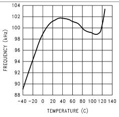
Figure 9. Oscillator Frequency vs Temperature
