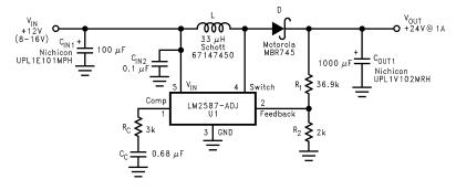
Figure 19. 12-V To 24-V Boost Regulator
