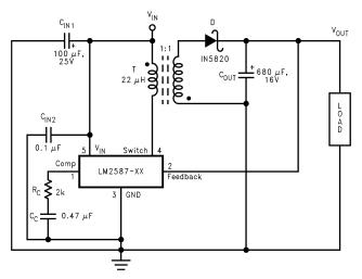
$C_{IN1}$ —100  $\mu F,$  25V Aluminum Electrolytic  $C_{IN2}$ —0.1  $\mu F$  CeramicT—22  $\mu H,$  1:1 Schott #67141450D—1N5820C\_OUT—680  $\mu F,$  16V Aluminum Electrolytic C\_C—0.47  $\mu F$  Ceramic R\_C—2k
