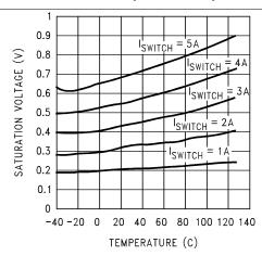
Figure 7. Switch Saturation Voltage vs Temperature
