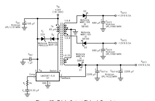
Figure 27. Triple-Output Flyback Regulator
