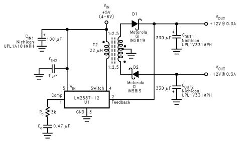
Figure 25. Dual-Output Flyback Regulator
