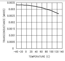
Figure 10. Error Amp Transconductance vs Temperature
