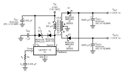
Figure 26. Dual-Output Flyback Regulator
