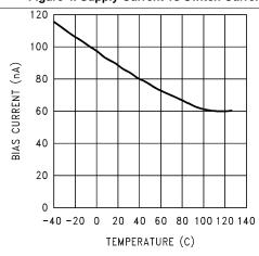
Figure 6. Feedback Pin Bias Current vs Temperature
