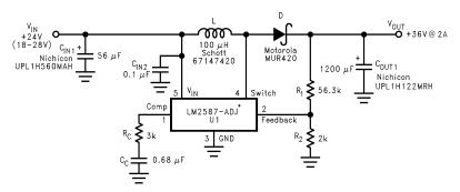
Figure 20. 24-V To 36-V Boost Regulator
