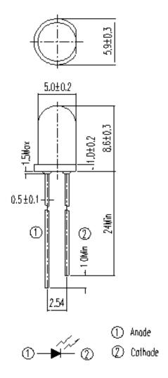
Note: Tolerances unless dimensions ±0.25mm
