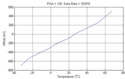
**Figure 6 Input Referred Offset Drift (Gain=128, Rate=10Hz)**
