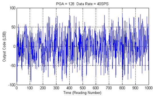
**Figure 3 Output Noise (Gain=128, Rate=40Hz)**
