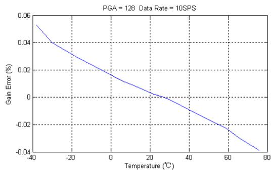
**Figure 7 Gain Drift (Gain=128, Rate=10Hz)**
