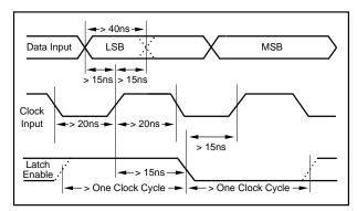
FIGURE 3. Setup and Hold Timing Diagram.
