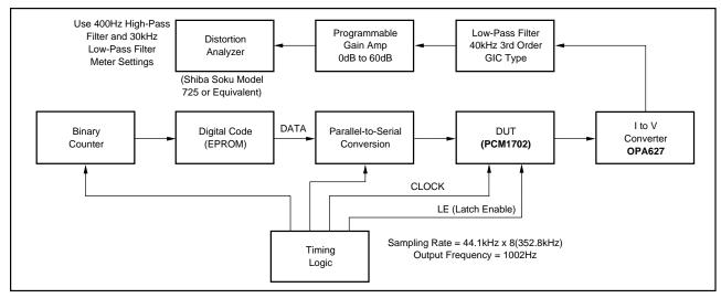
FIGURE 1. Production THD+N Test Setup.
