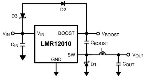
Figure 23. Zener Reduces Boost Voltage from  $V_{IN}$
