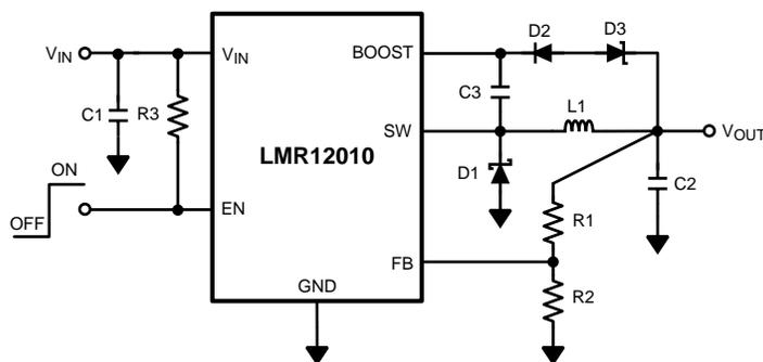
Figure 26.  $V_{BOOST}$  Derived from Series Zener Diode ( $V_{OUT}$ )
