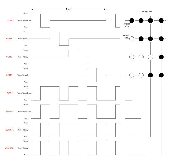
Waveforms for 1/4 Duty Drive Mode with 1/2 Bias ( $V_{\text{op}}=V_{\text{LCD}}-V_{\text{SS}}$ )
