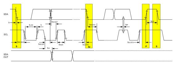
Note: The write cycle time  $t_{\text{WR}}$  is the time from a valid stop condition of a write sequence to the end of the valid start condition of a sequential command.
