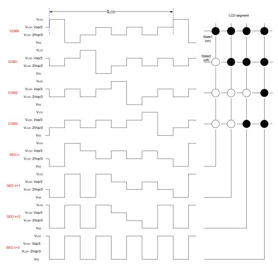
Waveforms for 1/4 Duty Drive Mode with 1/3 Bias ( $V_{\text{OP}}$ = $V_{\text{LCD}}$ - $V_{\text{SS}}$ )
