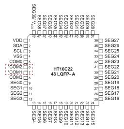
Note: The \*COM1 and \*COM2 pins are not in sequential order.
