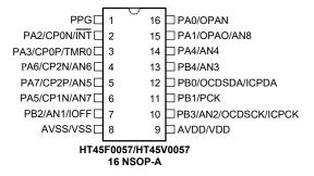
Note: The OCDSDA and OCDSCK pins are supplied for the OCDS dedicated pins and as such only available for the HT45V0057 device which is the OCDS EV chip for the HT45F0057 device.
