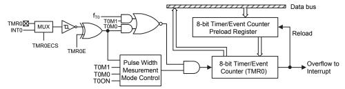
Note: INT0 is inverted or non-inverted de-bounce signal from  $\overline{\text{INT}}$  pin or comparator 0 output "C0VO" by software option.
