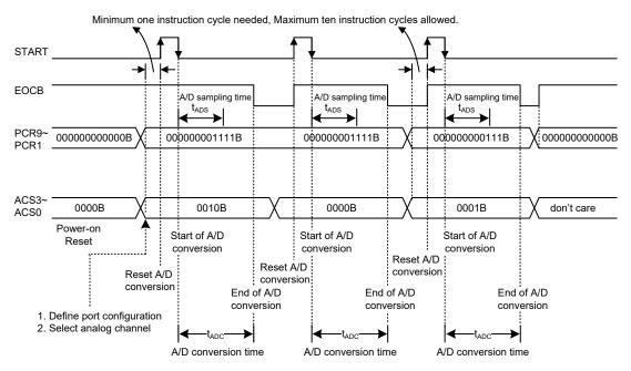
Note: A/D clock must be f\_SYS/2, f\_SYS/8 or f\_SYS/32  $t_{\text{ADCS}}\text{=}4t_{\text{ADCK}}$
