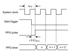
EX2: Since the first trigger type is raising edge after PPG starts, the PPG timer is triggered by raising edge until PPG stops.
