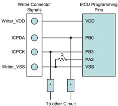
Note: 1.\* may be resistor or capacitor. The resistance of \* must be greater than  $1k\Omega$  or the capacitance of \* must be less than 1nF.
