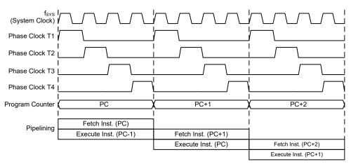
**System Clocking and Pipelining**
