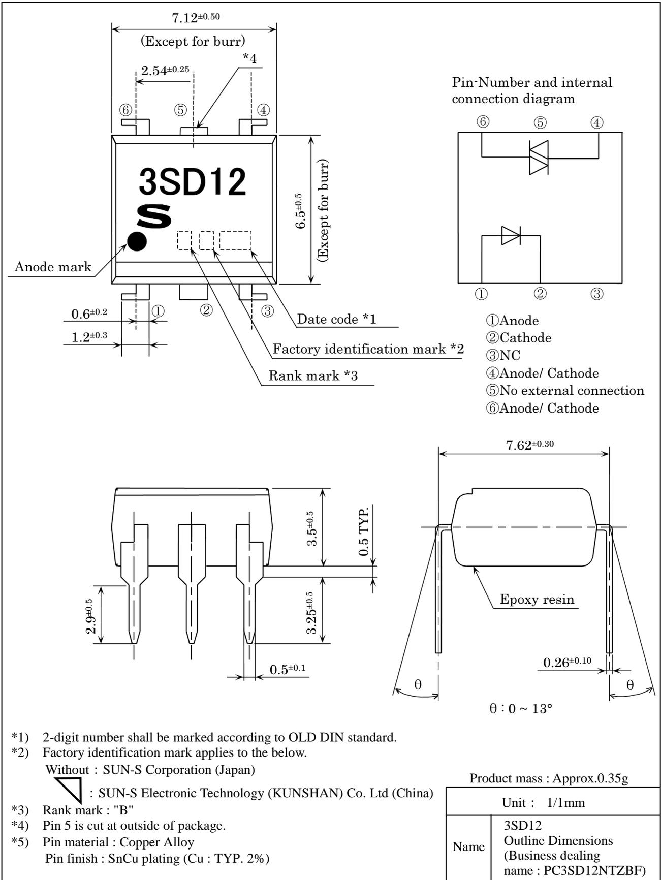
\*1) 2-digit number shall be marked according to OLD DIN standard.
