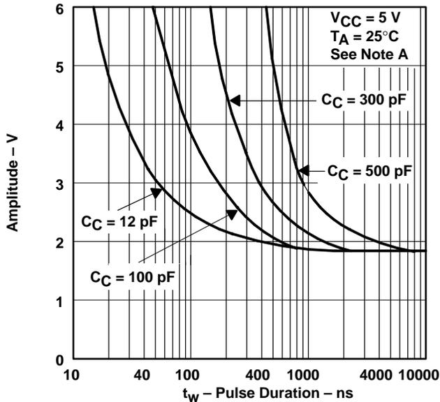
NOTE A: This figure shows the maximum amplitude of a positive-going pulse that, starting from 0 V, does not cause a change of the output level.
