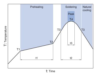
Preheating Soldering Peak Temp. Time Temp. Time Temp. Time T1 **T2** t1 Т3 t2 **T**4 t3 180°C 150°C 60 to 120s 10 to 30s 245°C 230°C 5s max. (4/7)
