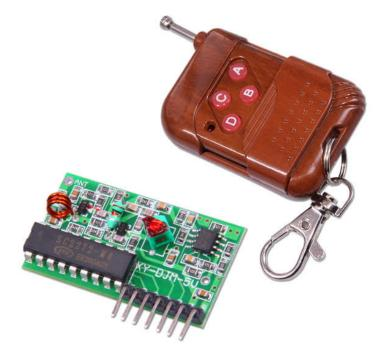
MX804 Remote Control Transmitter Power: 4.5~7V Quiescent Current (mA): 4.5 mA Modulation: AM (OOK) Operating Temperature: -10°C to +70°C Receiver sensitivity (dBm): -105 DB Operating range: up to 300m Channels: 4 Encoding: Encoding pad (fixed code)
