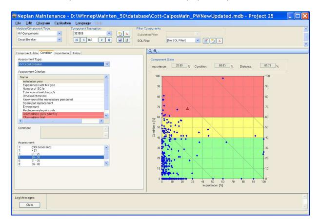
The condition of each component can easily be assessed with the freely configurable assessment sheets.
