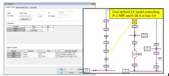
2) With the NEPLAN **function block drawing editor** the user may define graphically new dynamic models for controllers as well as for primary components and loads. The example on the right shows an exponential recovery load model.
