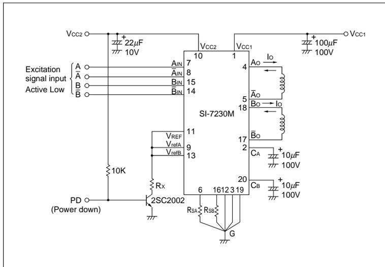
\* For details on the characteristics and thermal design, refer to the technical manual.
