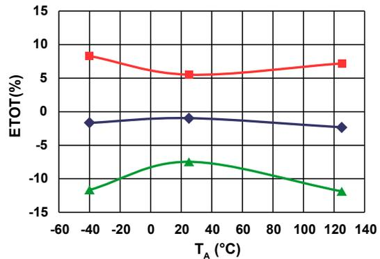
Symmetry versus Ambient Temperature
