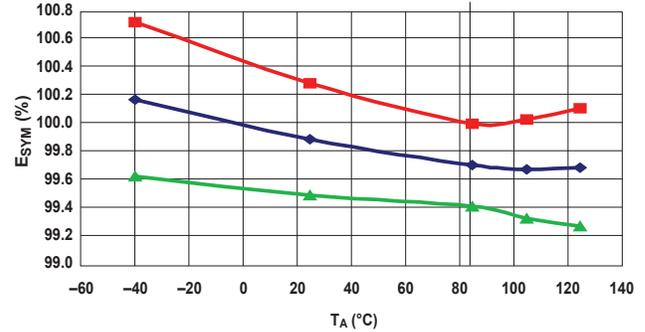
Total Output Error versus Ambient Temperature
