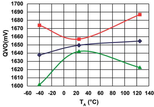
QVO Error versus Ambient Temperature
