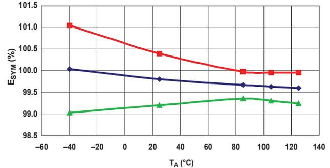
Total Output Error versus Ambient Temperature
