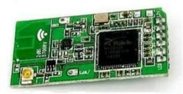
USB wifi module, built-in antenna, external, low power consumption, small size wireless module (Single-sided placement component)
