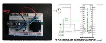
The display is connected by utilizing the i2c pins on your arduino.
