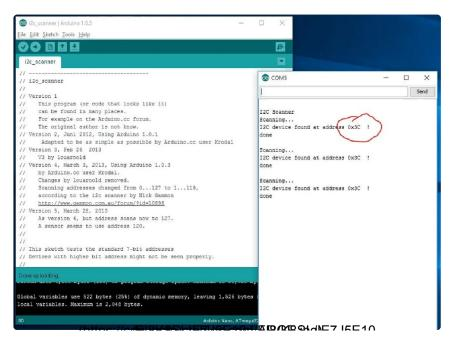
To start out, we need to find out the i2c address of the display. To
