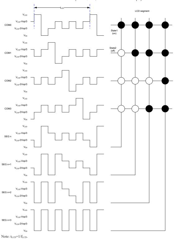
Waveforms for 1/4 Duty Drive Mode with 1/3 Bias ( $V_{\text{OP}}=V_{\text{LCD}}-V_{\text{SS}}$ )
