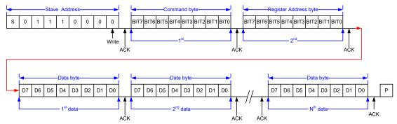
N Bytes Display RAM Data Write Operation
