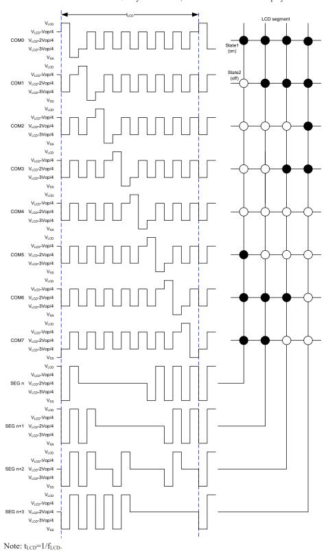
Waveforms for 1/8 Duty Drive Mode with 1/4 Bias (V<sub>OP</sub>=V<sub>LCD</sub>-V<sub>SS</sub>)
