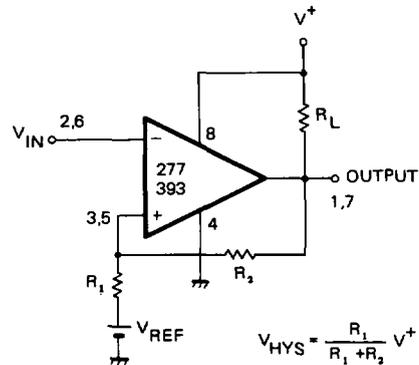
$$V_{HYS} = \frac{R_1}{R_1 + R_2} V^+$$
