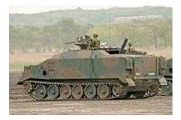
JGSDF Type 96 120 mm self-propelled mortar
