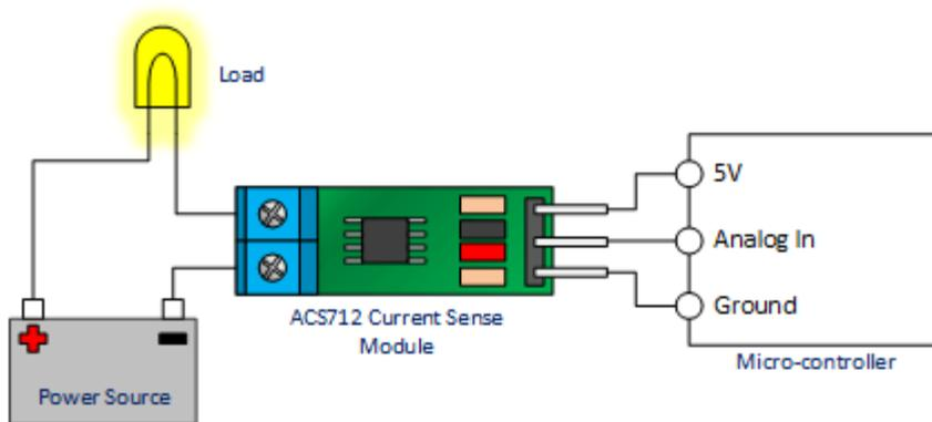
If the light bulb shown in the picture above were disconnected, the output of the ACS712 module would be 2.500 volts.
