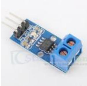
The ACS712 Current Sensors offered on the internet are designed to be easily used with micro controllers like the Arduino.
