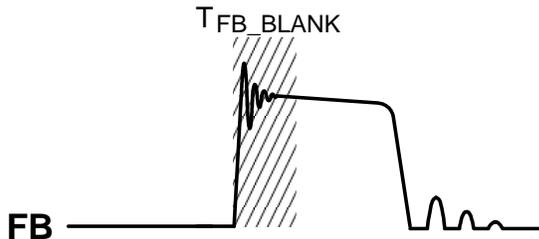
**Figure 4: Ringing waveform of FB voltage**
