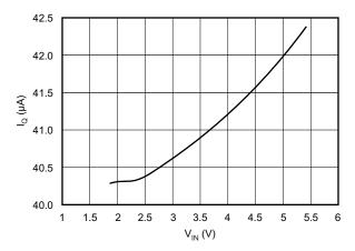
Figure 24. Supply Current vs Supply Voltage
