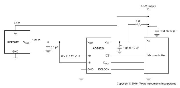
Figure 28. Basic Data Acquisition System 2
