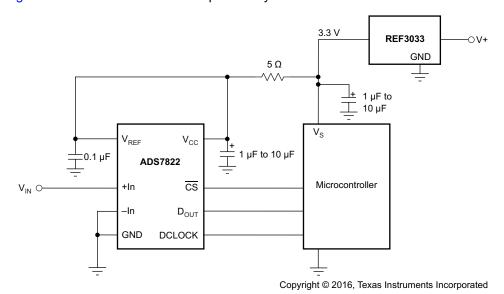
Figure 27. Basic Data Acquisition System 1
