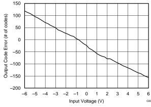
Figure 33. Output Code Error vs Input Voltage
