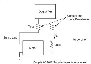
Figure 25. Accurate Load Regulation of REF30xx
