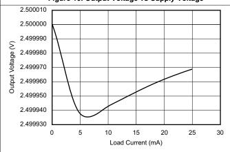
Figure 12. Output Voltage vs Load Current
