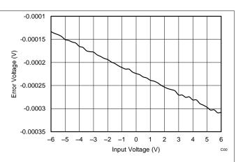
Figure 32. OPA317 Output Voltage Error vs Input Voltage
