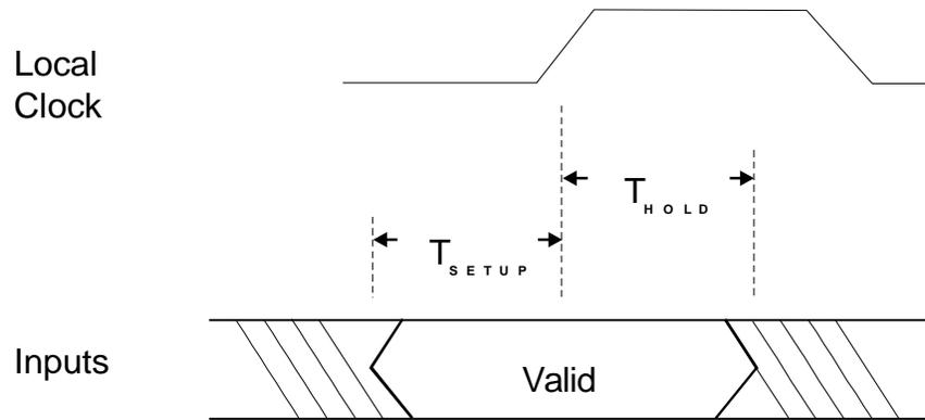
**Figure 6-2. PCI 9050 Local Input Setup and Hold Waveform****Table 6-6. Clock Frequencies**
