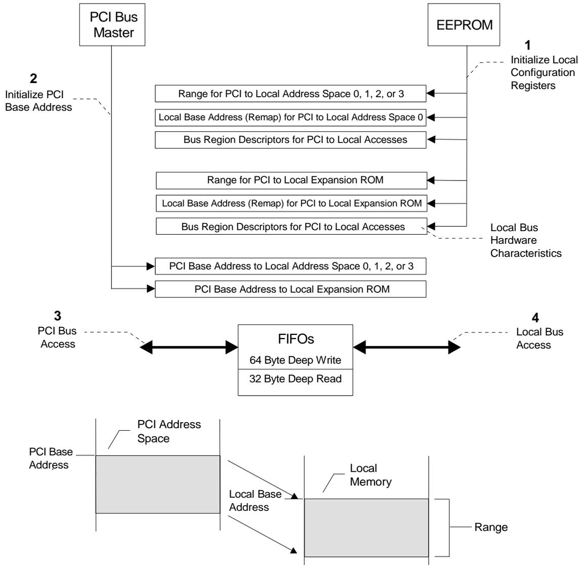
Figure 3-1. PCI Master Direct Access of Local Bus
