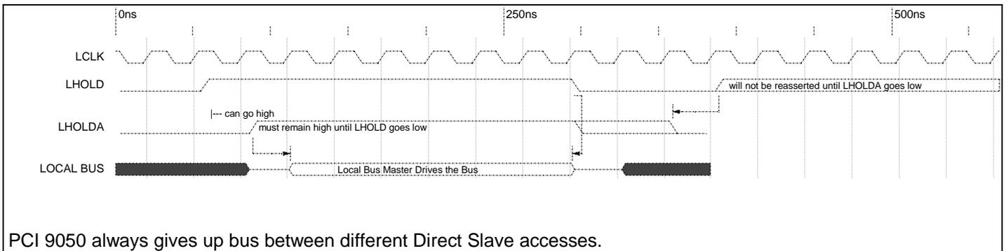
Timing Diagram 8-2. PCI 9050 Local Bus Arbitration
