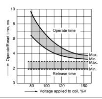
3.-(2) Set/Reset time (Latching) Sample: RK1-L-12V, RK1-L2-12V No. of samples: n = 12
