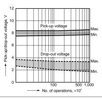
4.-(2) Mechanical life test (Latching) Sample: RK1-L2-12V No. of samples: n = 12
