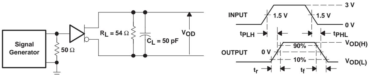
Figure 4. Driver Switching Test Circuit and Waveforms
