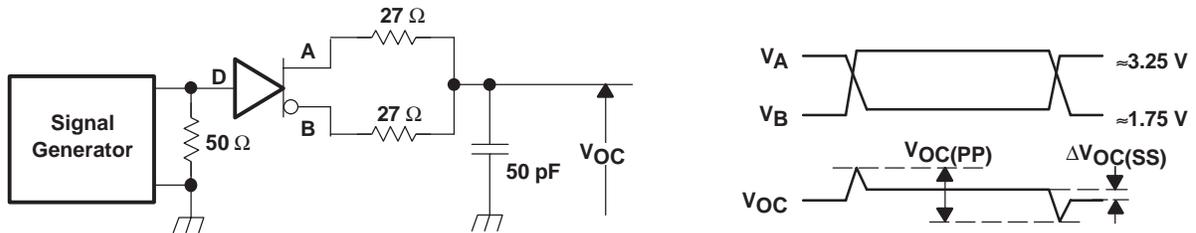
Figure 3. Driver  $V_{OC}$  Test Circuit and Waveforms
