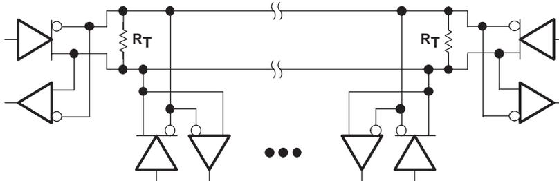
NOTE: The line should be terminated at both ends with its characteristic impedance ( $R_T = Z_0$ ). Stub lengths off the main line should be kept as short as possible.
