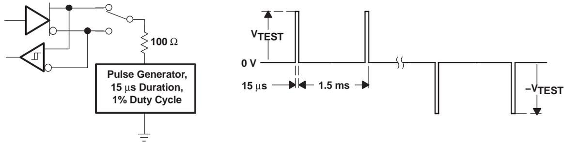
Figure 13. Test Circuit and Waveforms, Transient Over-Voltage Test
