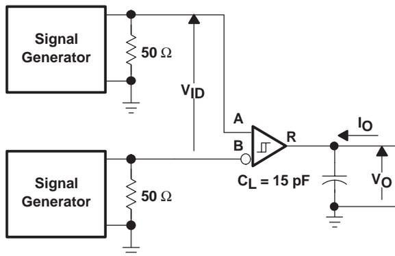
Figure 9. Receiver Switching Test Circuit and Waveforms
