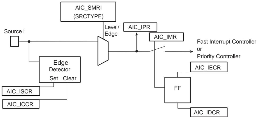
23.7.1.6 External Interrupt Source Input Stage
