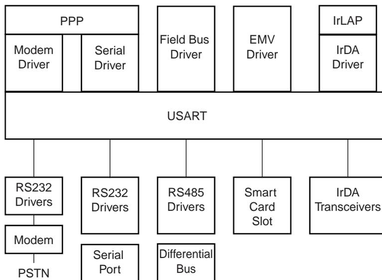
**Figure 31-4.** SAM7S32/16 Application Block Diagram
