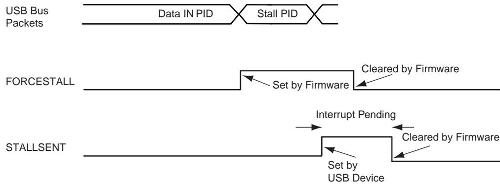
**Figure 35-13. Stall Handshake (Data OUT Transfer)**
