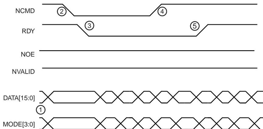
**Figure 20-4.** SAM7S32/16 Parallel Programming Timing, Write Sequence
