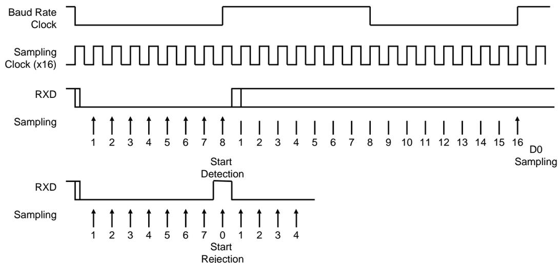
**Figure 31-11. Asynchronous Character Reception**
