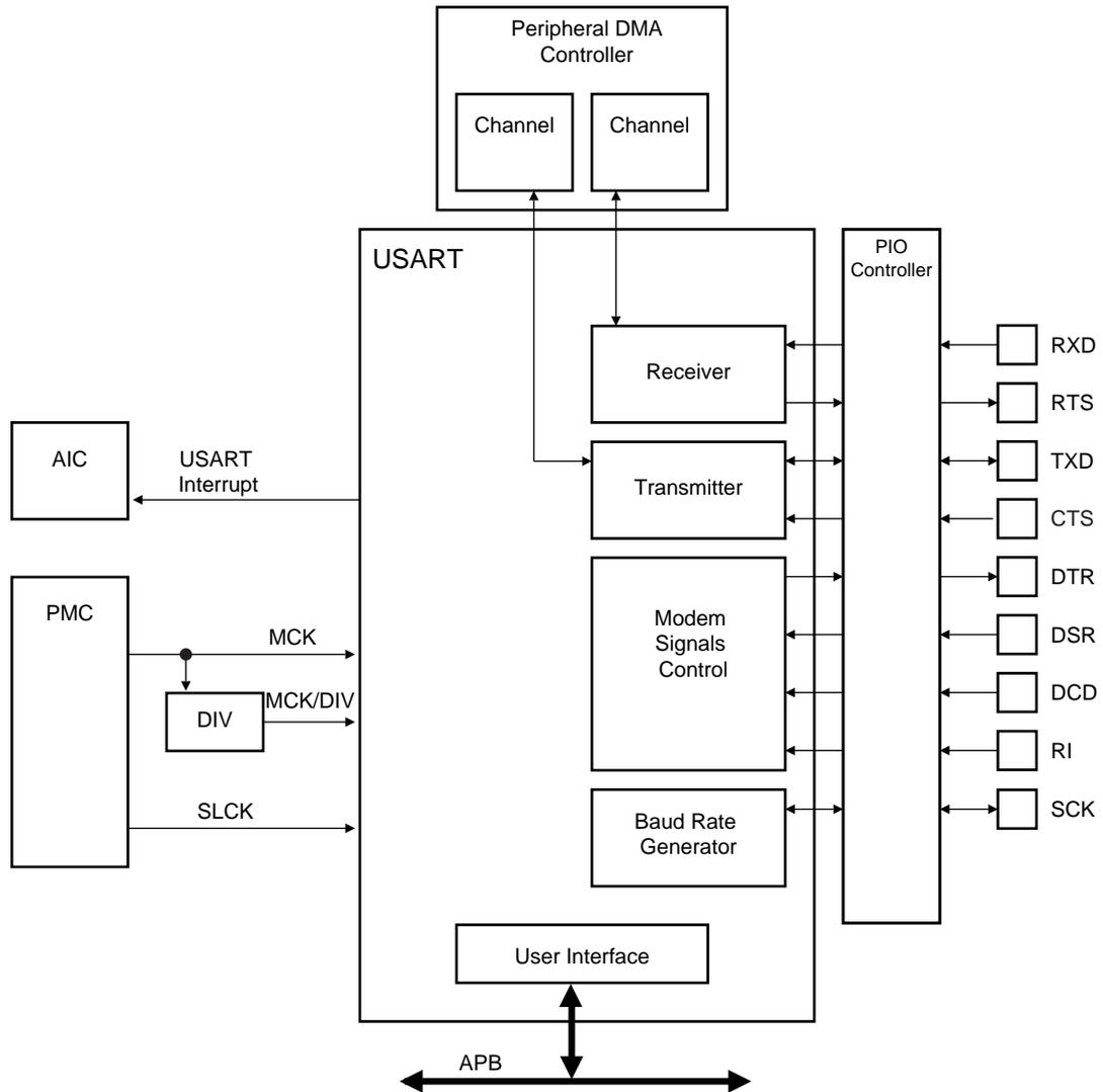
**Figure 31-2.** SAM7S32/16 USART Block Diagram
