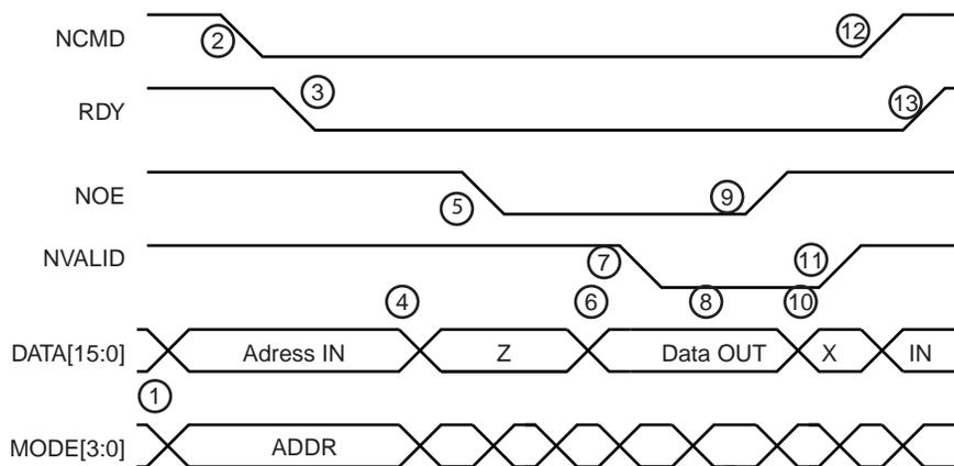
**Figure 20-6.** SAM7S32/16 Parallel Programming Timing, Read Sequence
