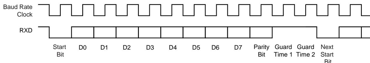
**Figure 31-24.**  $T = 0$  Protocol with Parity Error
