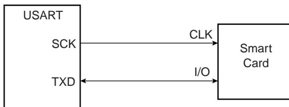
When operating in ISO7816, either in T = 0 or T = 1 modes, the character format is fixed. The configuration is 8 data bits, even parity and 1 or 2 stop bits, regardless of the values programmed in the CHRL, MODE9, PAR and
