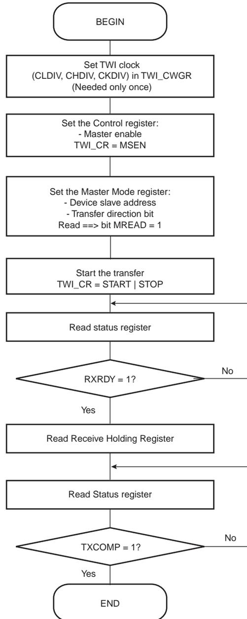
Figure 29-17. TWI Read Operation with Single Data Byte and Internal Address
