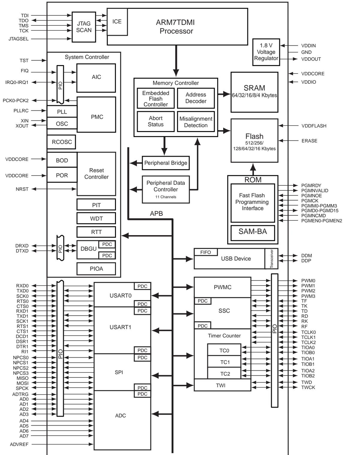
Figure 2-2. SAM7S32/16 Block Diagram
