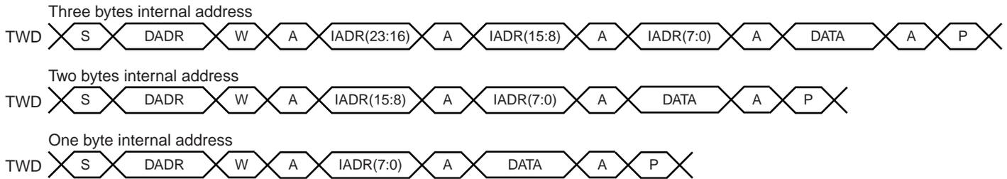
**Figure 30-12. Master Read with One, Two or Three Bytes Internal Address and One Data Byte**
