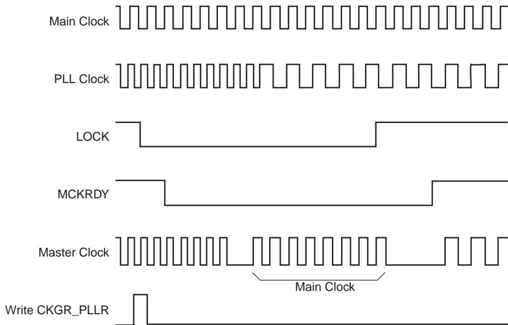
**Figure 25-6.** Programmable Clock Output Programming
