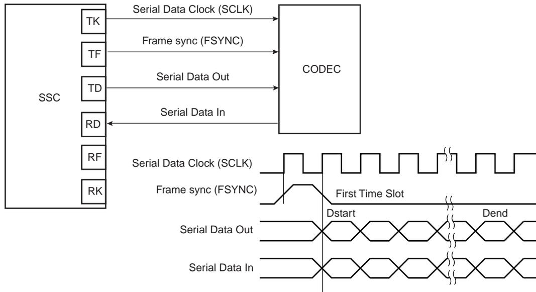
**Figure 32-19.** Time Slot Application Block Diagram
