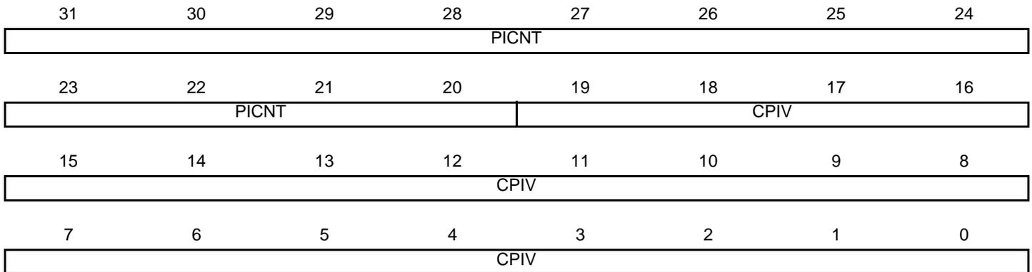
Reading this register clears PITS in PIT\_SR.
