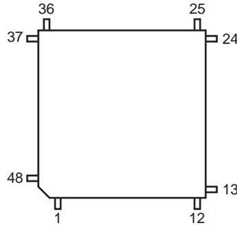
Figure 4-4. 48-pad QFN Package (Top View)
