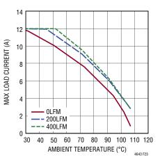
Figure 23. 12V<sub>IN</sub> to 3.3V<sub>OUT</sub> Derating Curve, 4-Channel Paralleled, No Heat Sink
