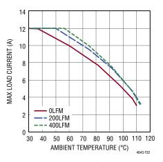
Figure 22. 5V<sub>IN</sub> to 3.3V<sub>OUT</sub> Derating Curve, 4-Channel Paralleled, No Heat Sink
