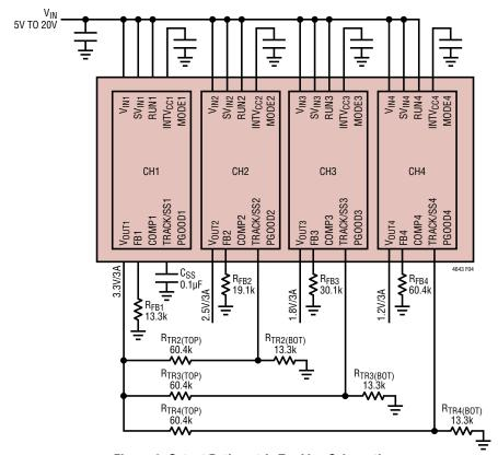
Figure 4. Output Ratiometric Tracking Schematic
