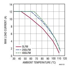
Figure 21. 12V<sub>IN</sub> to 1.5V<sub>OUT</sub> Derating Curve, 4-Channel Paralleled, BGA Heat Sink
