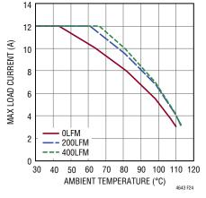
Figure 24. 5V<sub>IN</sub> to 3.3V<sub>OUT</sub> Derating Curve, 4-Channel Paralleled, BGA Heat Sink
