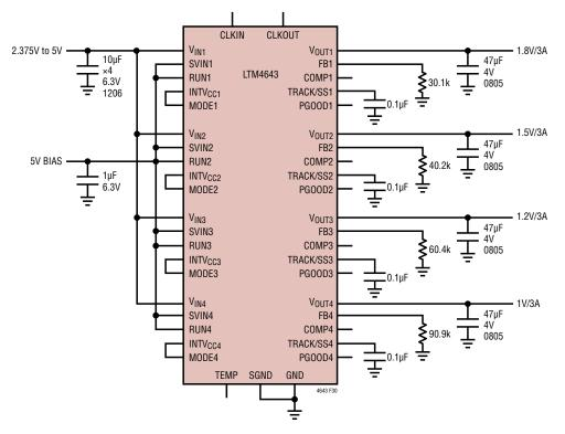
Figure 30. 2.375V to 5V Input, Quad 1V, 1.2V, 1.5V, 1.8V Output
