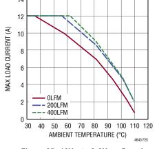
Figure 25. 12V<sub>IN</sub> to 3.3V<sub>OUT</sub> Derating Curve, 4-Channel Paralleled, BGA Heat Sink
