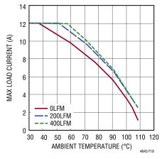
Figure 19. 12V<sub>IN</sub> to 1.5V<sub>OUT</sub> Derating Curve, 4-Channel Paralleled, No Heat Sink
