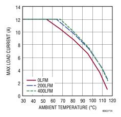
Figure 14. 5V<sub>IN</sub> to 1.0V<sub>OUT</sub> Derating Curve, 4-Channel Paralleled, No Heat Sink
