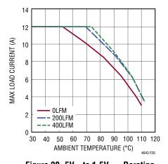
Figure 20. 5V<sub>IN</sub> to 1.5V<sub>OUT</sub> Derating Curve, 4-Channel Paralleled, BGA Heat Sink
