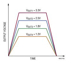
Figure 3. Output Ratiometric Tracking Waveform
