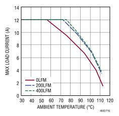
Figure 16. 5V<sub>IN</sub> to 1.0V<sub>OUT</sub> Derating Curve, 4-Channel Paralleled, BGA Heat Sink
