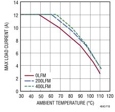
Figure 18. 5V<sub>IN</sub> to 1.5V<sub>OUT</sub> Derating Curve, 4-Channel Paralleled, No Heat Sink
