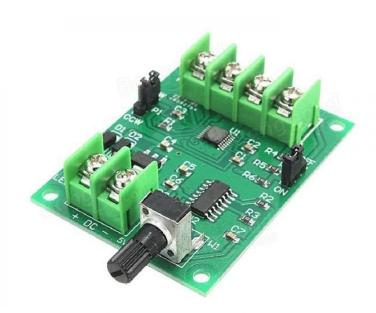
The driver board can drive hard disk brushless motors, CD-ROM brushless motors and other micro brushless motor of line 3 or 4 wires without hall sensor.. It has the reverse voltage protection, over current protection to ensure the usage safety. The driver voltage 5-12V, the higher the voltage the faster the speed, the maximum speed up to 10,000rpm.
