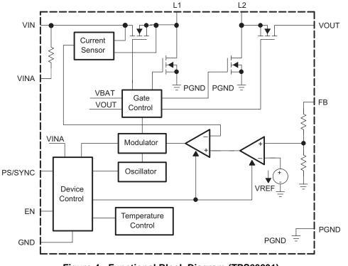
Figure 4. Functional Block Diagram (TPS63031)
