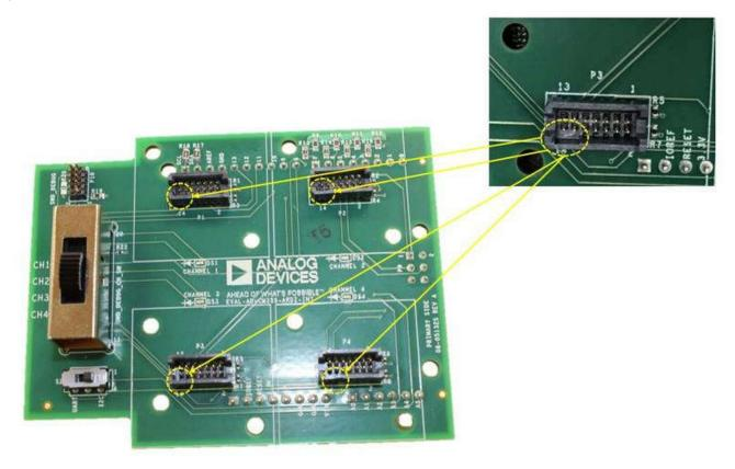
Check if connectors P1, P2, P3 and P4 were correctly installed. The notch found for all header should be at the bottom left near the header number 14 of the silk screen.
