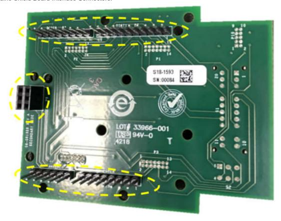
Pictured above is the EVAL-M355-ARDZ-INT interposer board which was developed to quickly and easily connect ADICUP3029 development board or any equivalent Arduino MCU controller boards.
