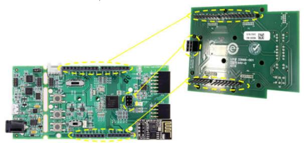
4. Placed on the desired number of ADuCM355 sensor daughter board on top of the interposer board.(up to 4)
