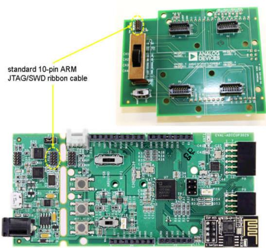
There is a way to cut the SWD traces on the ADICUP3029 board right at the break away section of the board. By cutting the trace for the SWD\_DIO, SWD\_CLK and SWD\_RST located near P12. There are two(2) traces on the top of the board that must be cut using a knife, and one(1) trace found at the bottom of ADICUP3029 (the outter most trace), This allows customers to program both the ADICUP3029 and M355-INT boards without losing the ability to stream serial data back to the USB port.
