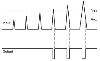
Figure 33. Threshold Detector
