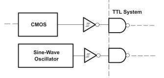
Figure 30. TTL System Interface For Slow Input Waveforms
