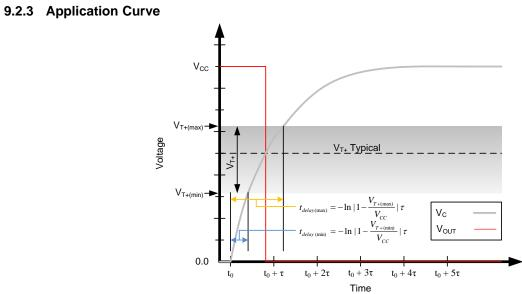
Figure 29. Ideal Capacitor Voltage and Output Voltage With Positive Switching Threshold
