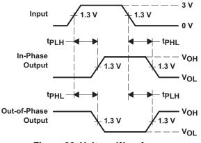
Figure 26. Voltage Waveforms Propagation Delay Times
