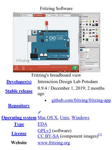
**Fritzing** is an <u>open-source</u> initiative<sup>[2]</sup> to develop amateur or hobby <u>CAD software</u> for the <u>design</u> <u>of electronics hardware</u>, to support designers and artists ready to move from experimenting with a prototype to building a more permanent circuit. It was developed at the <u>University of Applied</u> <u>Sciences Potsdam</u>.<sup>[3]</sup>
