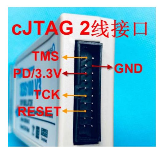
cJTAGRequired pins: 1,TCK (Downloader11foot) 2,TMS (Downloader1foot) 3,3.3V (Downloader5foot) 4, GND (Downloader4foot) 5,RESET (Downloader15foot)
