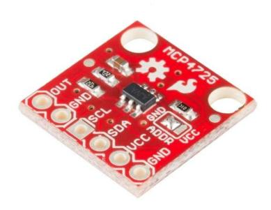
The MCP4725 is an I<sup>2</sup>C controlled Digital-to-Analog converter (DAC). Digital to analog converters are great for sound generation, musical instruments, and many other creative projects!
