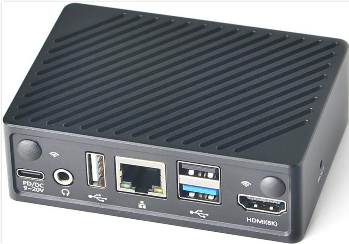
Image 2.1: Front view of the NanoPi M6, showing USB-C power, audio jack, USB 2.0, Gigabit Ethernet, USB 3.0, and HDMI ports.
